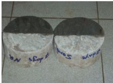
Figure 5. Rapid chloride permeability test
