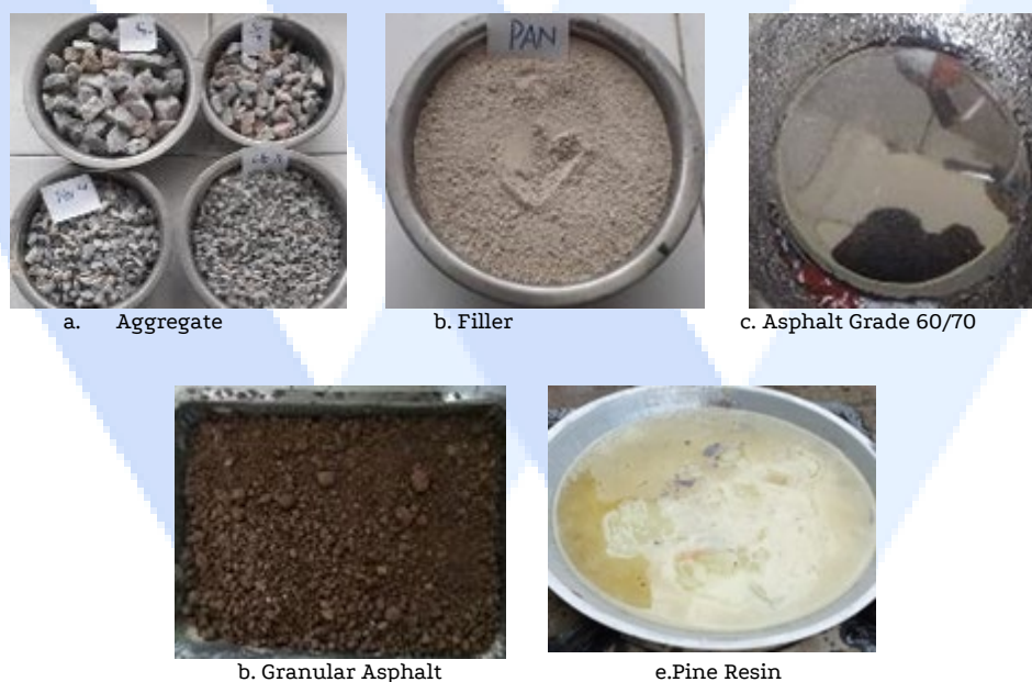
Figure 1. Materials used to make specimens of hot mix asphalt AC-WC
