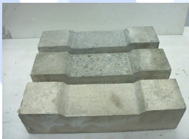
Figure 3. Beams for Flexural test
