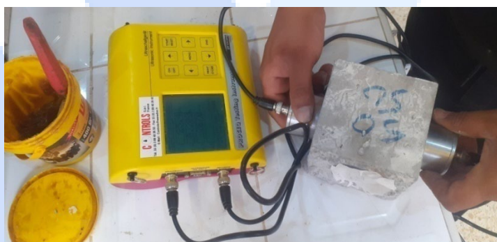
Figure 9. Calibrating the Ultrasound device
