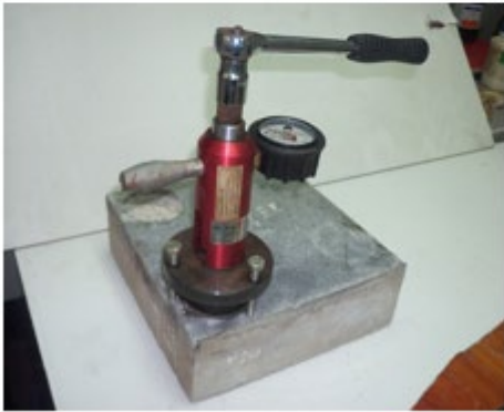
Pull off test
