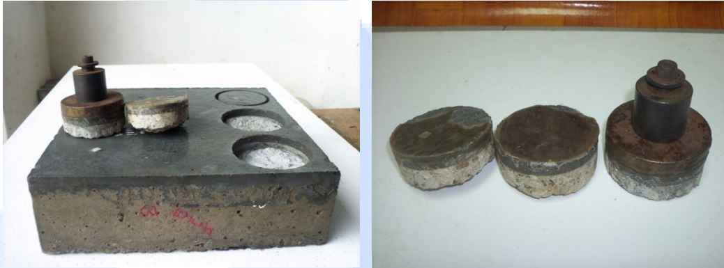
Figure 19. (a) Pull off test set-up for the composite specimen, (b) Failure through the NC substrate
