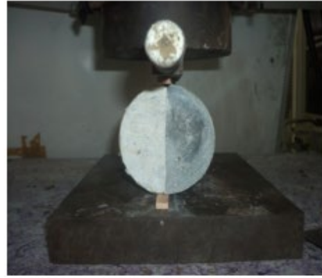
Splitting tensile test
