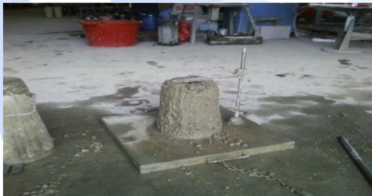
Figure 7. Concrete slump measurement at Abrams cone
