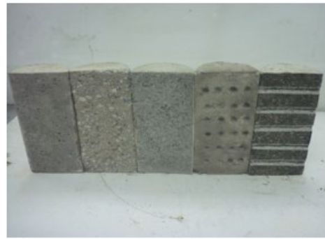
Halved longitudinal cylinder for Splitting tensile test
