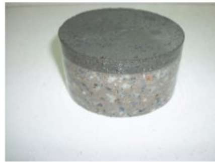
Figure 5. Rapid chloride permeability test
